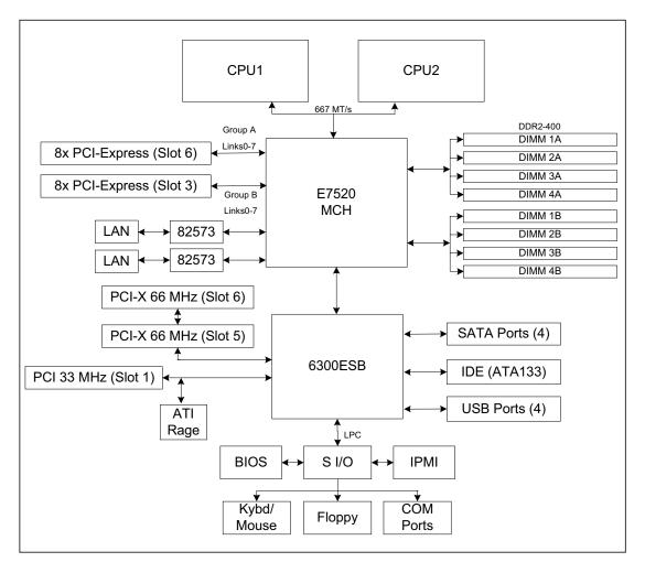
Figure 1-1. Intel E7520 Chipset: System Block Diagram
